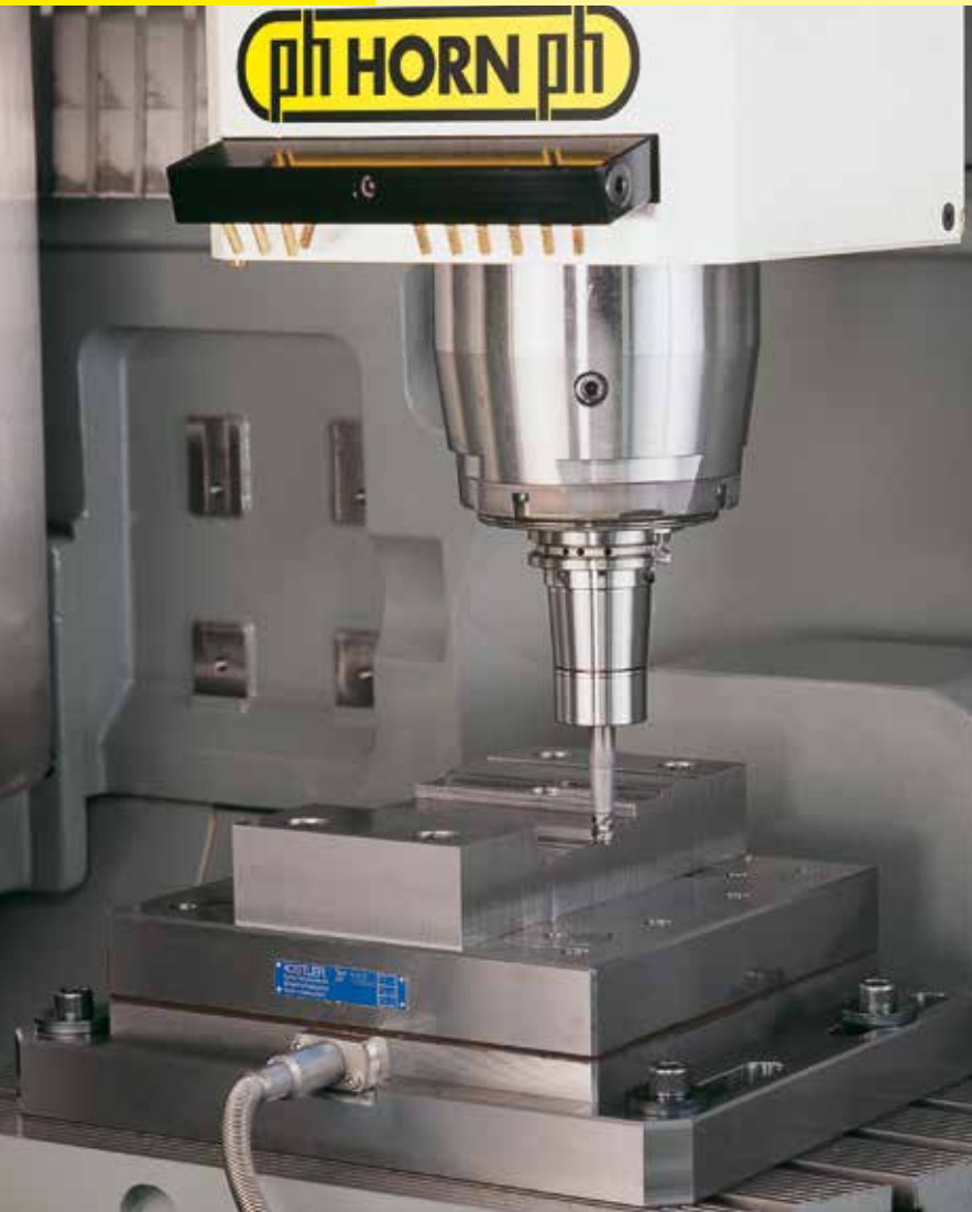
Test set up for measuring the radial and axial forces on a solid carbide endmill using a three component measuring platform.
