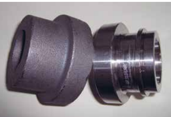
Forged Blank and ready machined workpiece
