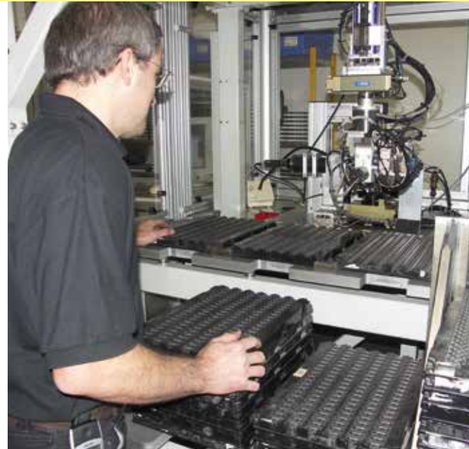
Automatically operating measurement machines check each carbide insert for dimensional accuracy.
