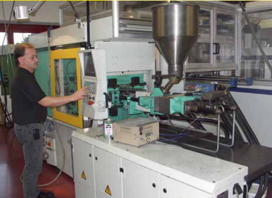
The carbide mixture is injected in a mould during injection moulding. After opening the mould, a gripper removes the blank and deposits it on a graphite plate.
