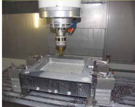
The 230 x 250 mm (9.055" x 9.843") pocket of an injection moulding tool is first rough milled dry (left picture) to 5 mm (0.197") and then rough milled wet to 44 mm (1.732") depth (right picture) with a 32 mm (1.26") diameter DAH milling cutter.
