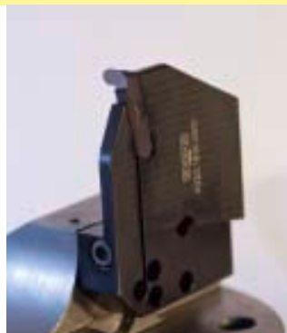
Cassette K220 with hook-shaped insert S229. A Trevisan basic holder is used as a tool holder.
