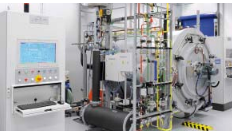
View of one of the fully automated pre-sintering furnaces.
