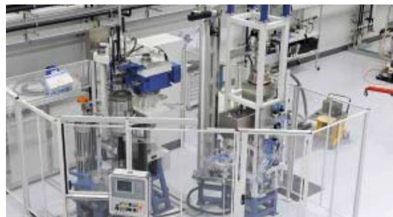
Isostatic press (left) and filling tower (right).
