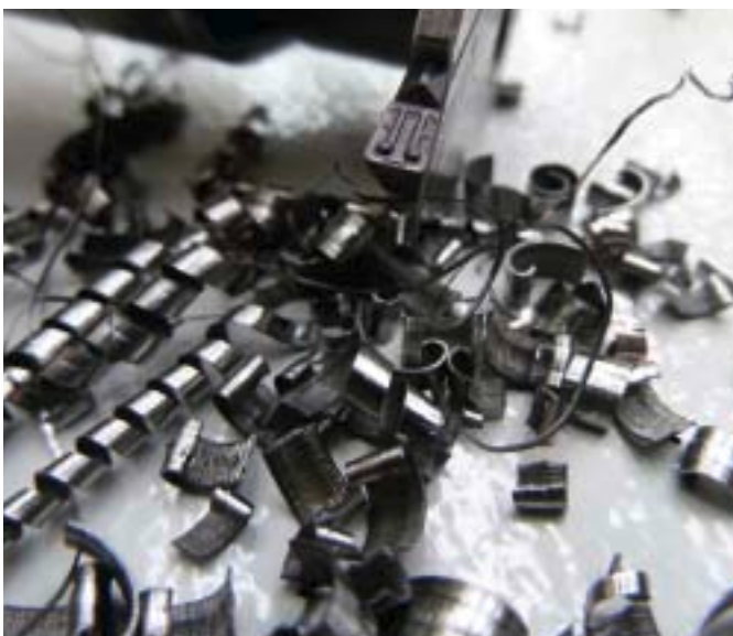
The L geometry ensures reliable chip break during internal grooving.
