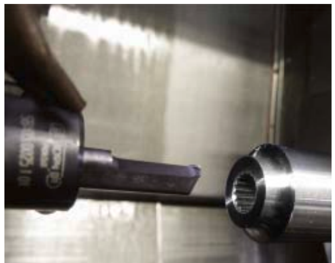
The teeth of the internal toothing are broached to a tooth profile depth of 0.6 mm (0,024") with a type 105 special plate in three infeeds.
