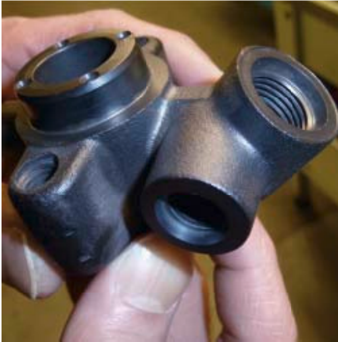
Guide piece for a suspension cylinder, a component with several precise internal contours.
