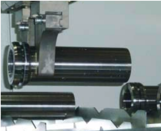
Automatic gripper on the gantry. Adhering chips must not be pressed into the high-quality surface during gripping.
