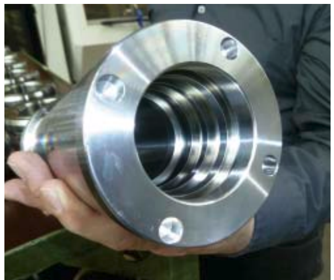
Four internal grooves for guide and sealing rings.
