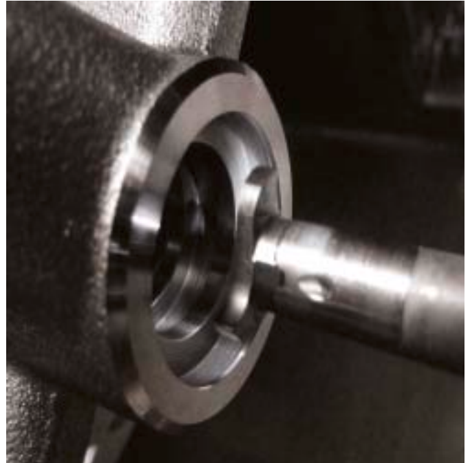
Rough milling is performed with a type 308 circular milling cutter with long throat depth.
