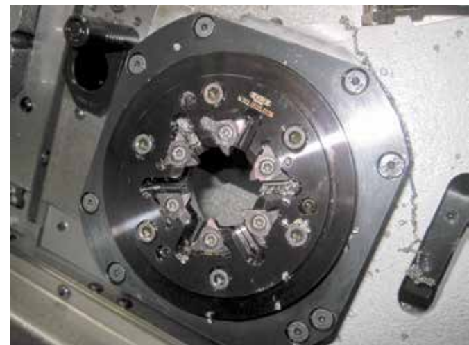
Whirling head type M302 with 6 cutting edges fixed on the whirling unit of the lathe
