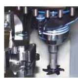
Picture, top: The slots are milled in the two jaw sections with the slot miller 636.
