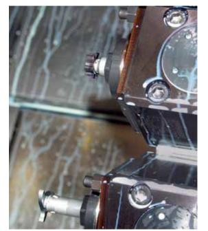
HORN milling tools in the turret of the lathe.
