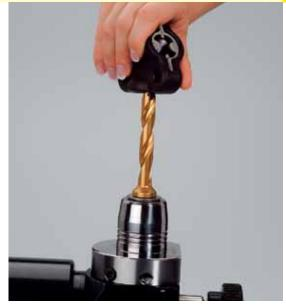
Simple and high-precision head replacement due to centre bore in the main body and stud in the carbide head: Insert head, turn slightly (picture left) and fix with key (picture right).
