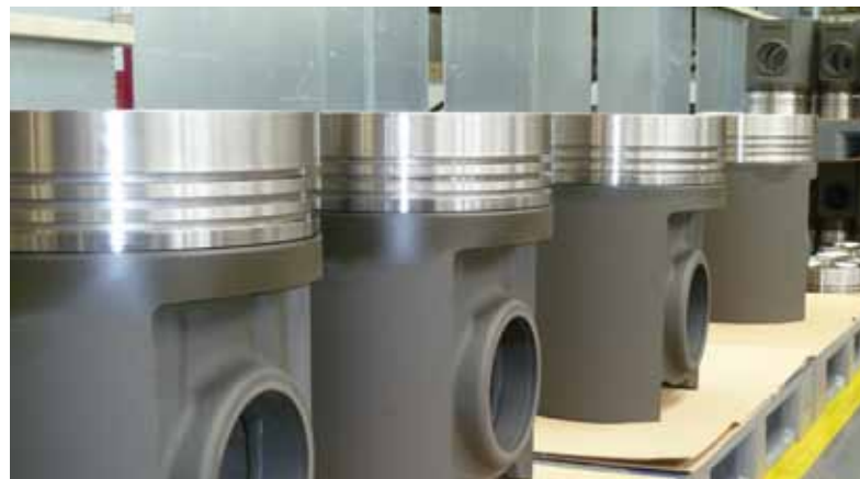
The partnership between KS Kolbenschmidt and HORN for machining piston ring grooves for large-bore pistons led to the development of the high-pressure internal cooling system.
