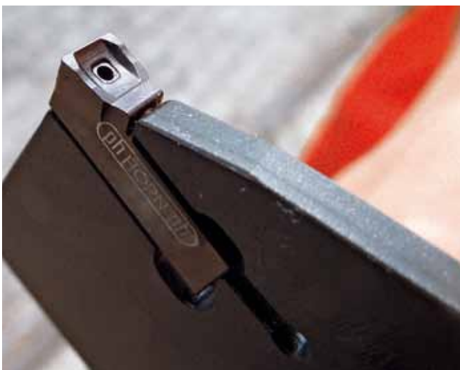
The special geometry of the nozzle shape ensures optimal cooling and chip removal as well as long tool lives for the cutting inserts.
