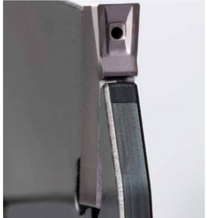
No steam bubbles: coolant comes straight out of the S100 chip surface with internal cooling.
