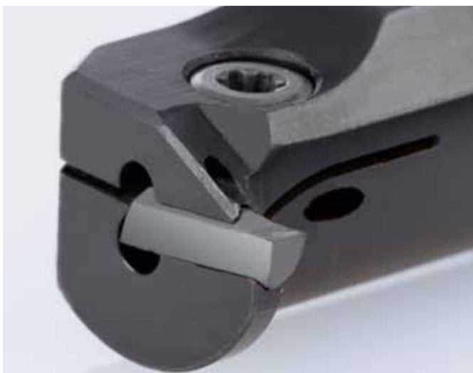
Coolant supply via clamping finger and additional bore in shank/neck for maximum tool life and effective chip transport.
