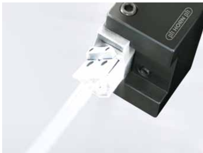
Cryogenic cooling. Liquid nitrogen can be used in cutting applications.
