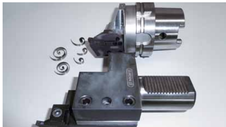
Two systems with internal cooling: The HSK 100 main body with cassette system is adapted to the turning/drilling/milling unit; the VDI holder to the turret. Both ensure short, controlled chips.
