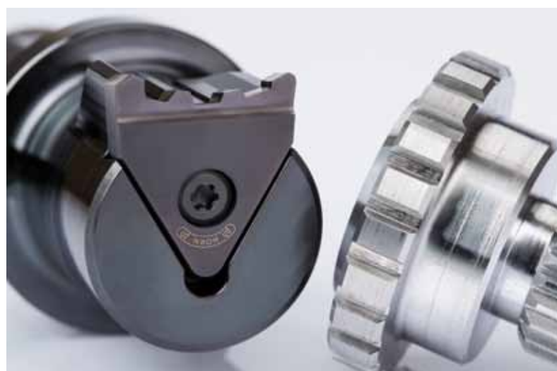
Gear broaching tool SH117 with pre-cutting and finishing profile to allow simultaneous pre-broaching and finishing of the gear.
