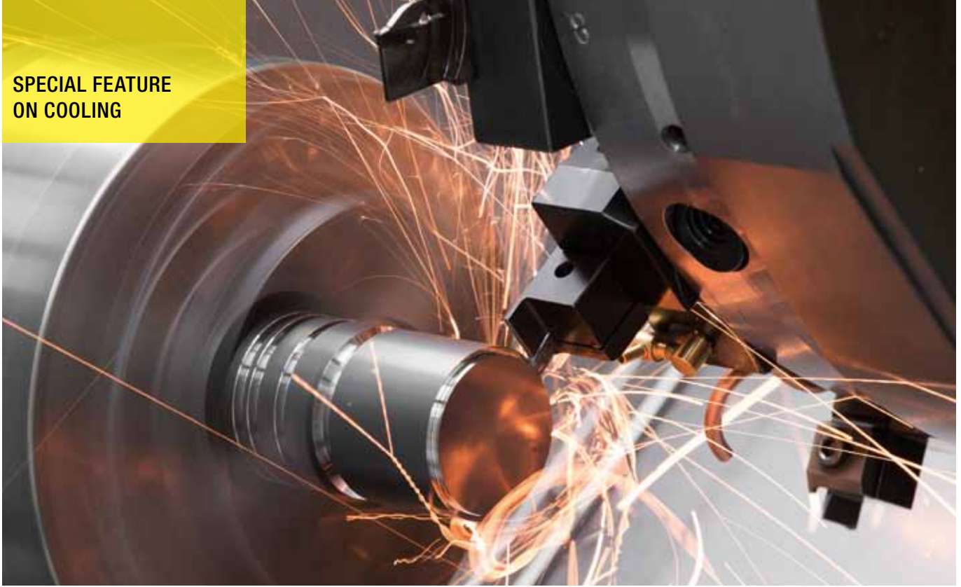
CBN hard turning during dry machining.
