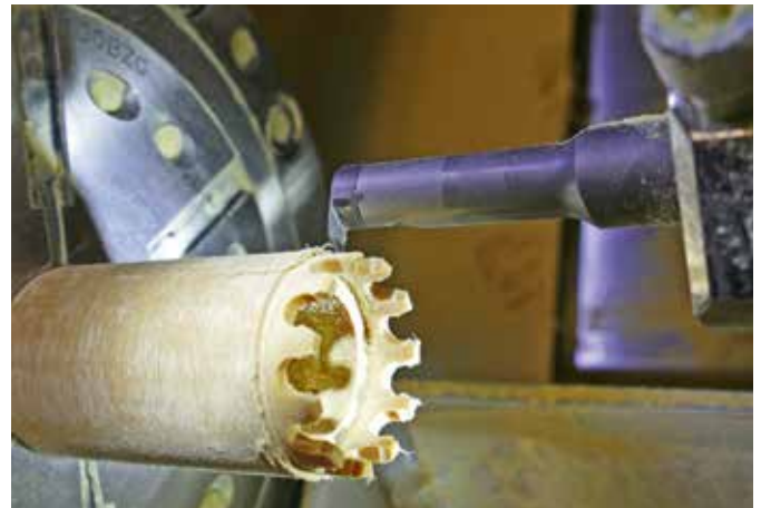
Parting off the ball-bearing cage with a special tool from the "Mini" range, type 18P, from HORN. The cutting material of the 1 mm (0.0394") wide tool consists of CVD thick-film diamond.
