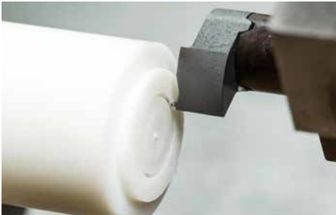
Axial grooving with HORN type 114 with PCD cutting edge in pure, off-the-shelf PTFE. Optimum surface quality and no burr formation.
