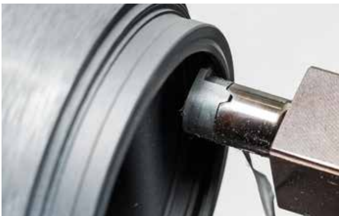
Small and medium-sized sealing rings are machined from the pipe. Shown in image: machining an interior contour using the HORN type 114 with PCD cutting edge.
