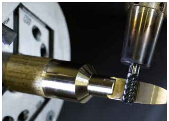
Rough milling (image 1), groove milling by circular interpolation (image 2) and finish milling (image 3): lead-free brass, like almost any material, offers a wide spectrum of possible machining operations.
