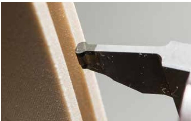
Cutting insert for manufacturing the entire interior contour of a PTFE seal using a PCD cutting edge. Whereas previously the interior contour had to be mapped out using several special carbide die plates, today just one PCD die plate is required.
