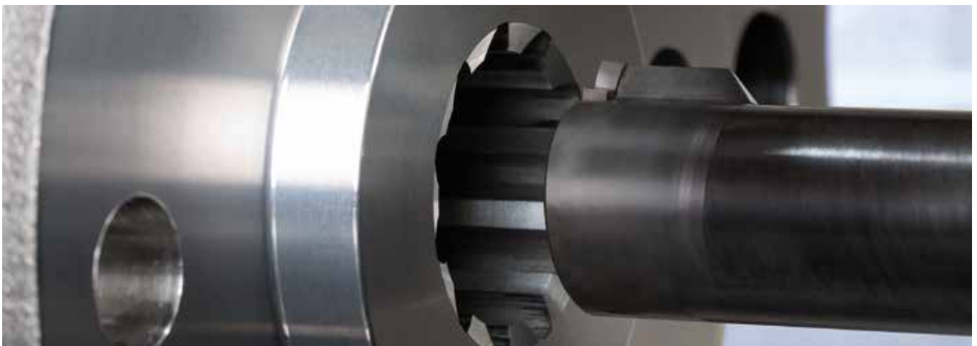
The S117 tool is in 12 o'clock position when broaching internal gear teeth.
