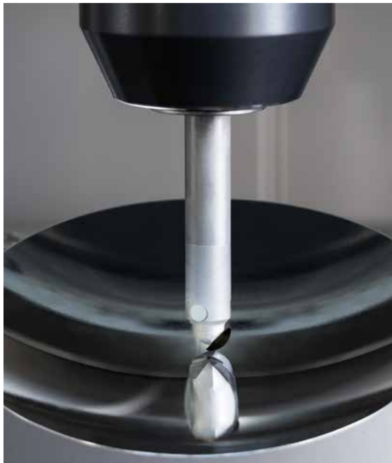
Mirror-finish milling of the concave mirror surface with vibration-damping carbide shaft from the type 117 range and 10 mm cutting insert type S117 with monocrystalline diamond cutting edge.
