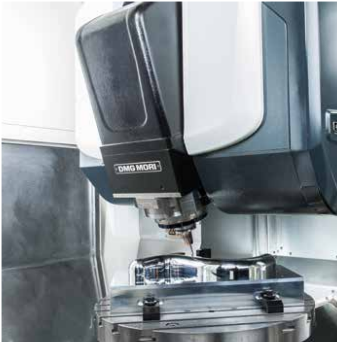
The thermosymmetrical construction of the HSC 70 linear ensures high precision brilliant-finish machining.
