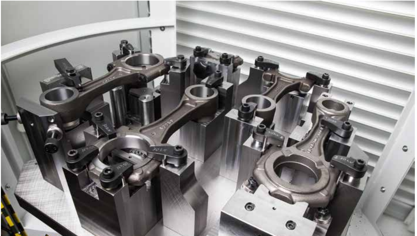
The connecting rods are machined in five stages. Machining starts on the right hand rod with the milling of the eye surfaces.
