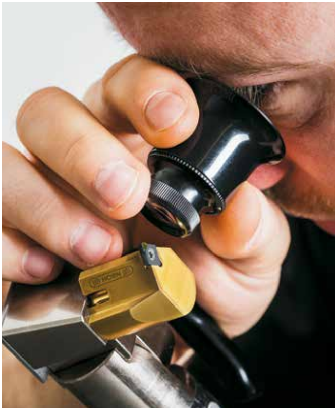
Absolutely vital: the visual inspection of a ground MCD cutting insert.
