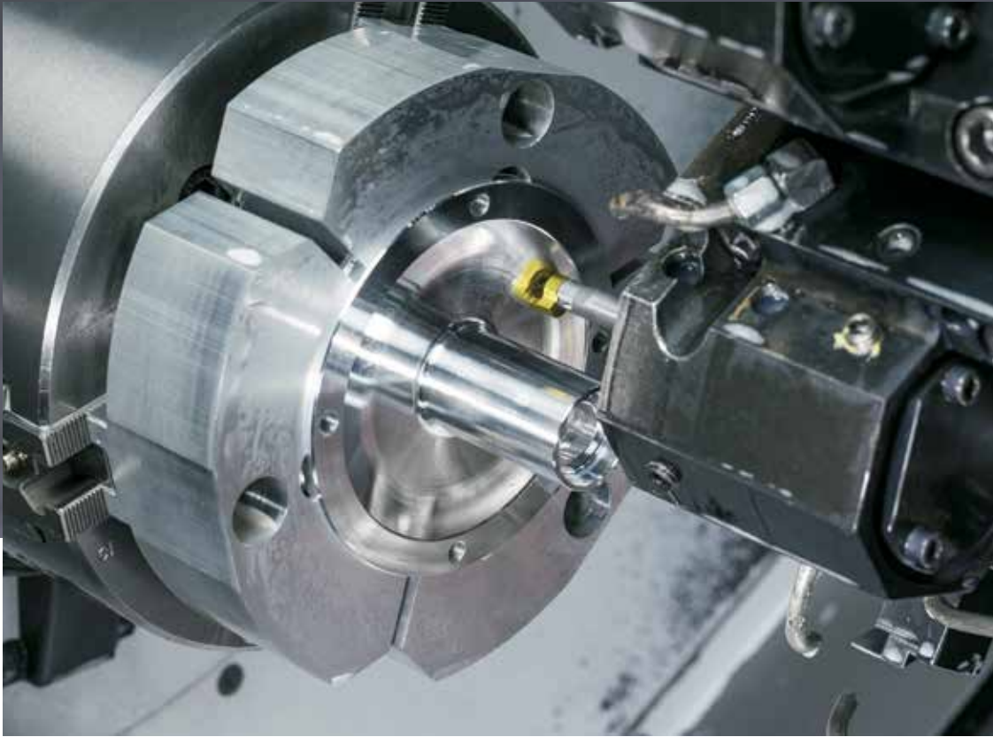
Finishing the small outside diameter and the concave face with the Mini R114 axial grooving tool.
