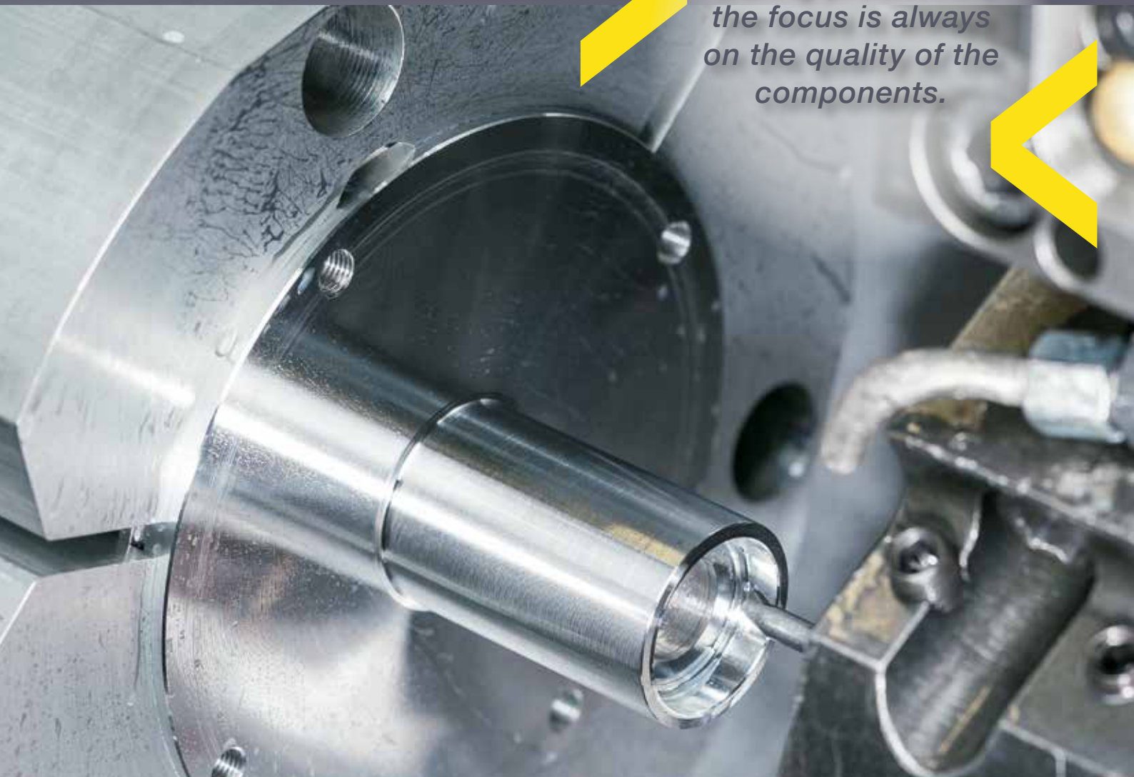
Boring an internal diameter with the Supermini system, type 105.
