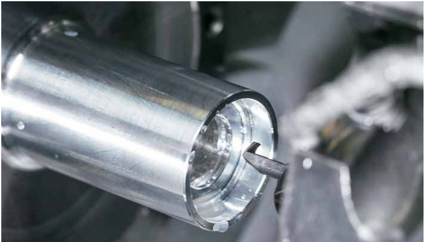
Supermini type 105 being used to machine a 1 mm (0.0394") wide internal groove.
