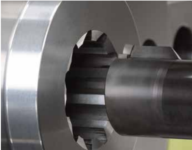
Always broach in a 12 o'clock position and program a lifting and feeding radius that will not harm the machinery.
