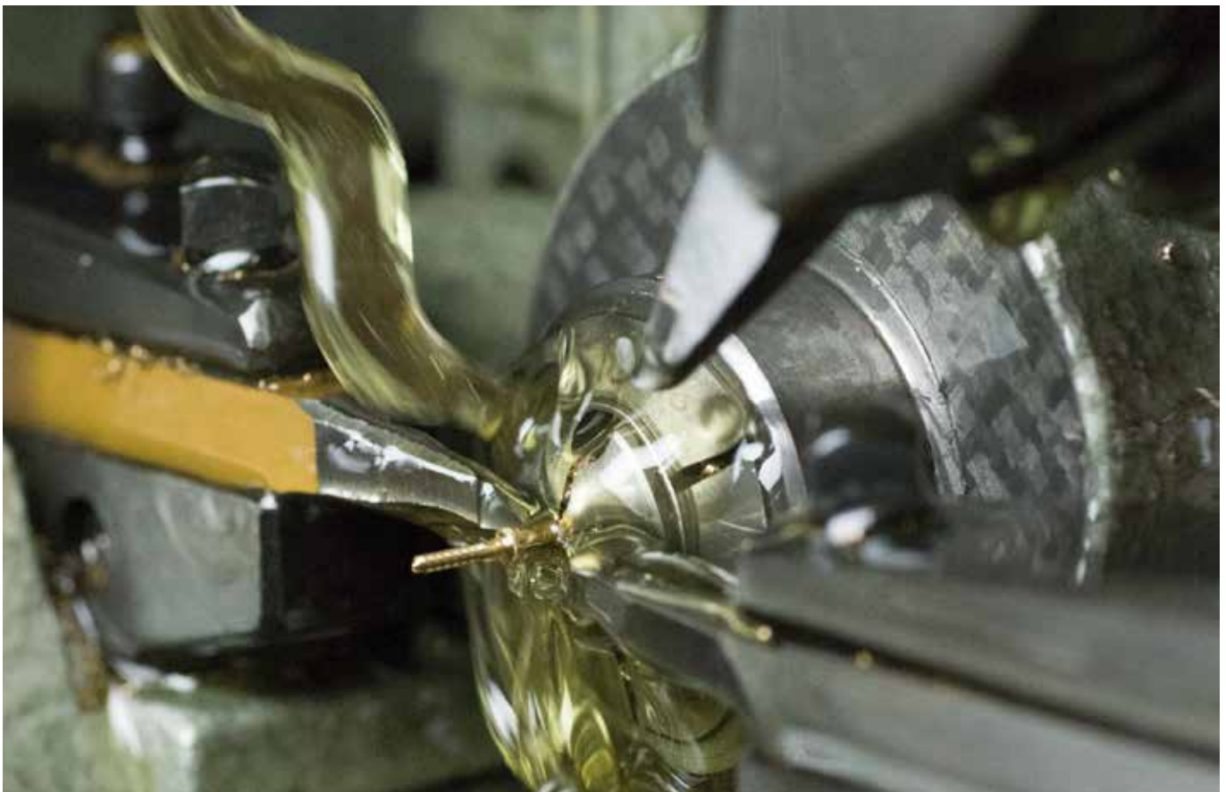
Screws, shafts and other components with exceptionally small diameters require special machine concepts and tool solutions.
