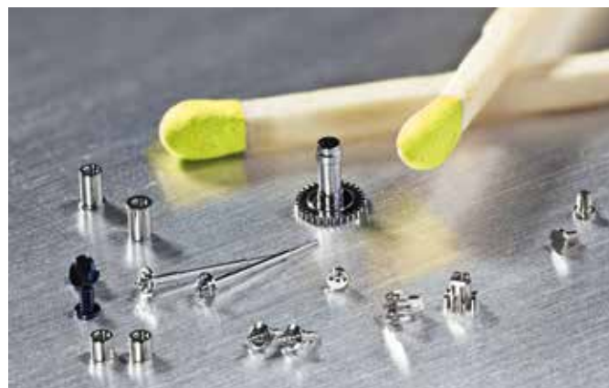
Accurately micro-machining shafts, tiny screws, sleeves and gear wheels on a micro-unit scale, while maintaining the very highest standards of surface quality, requires precision cutting tools.
