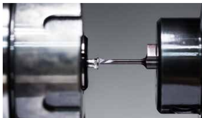
The multifaceted precision tool that Damasko uses to machine many of its watch components: the Supermini 105.
