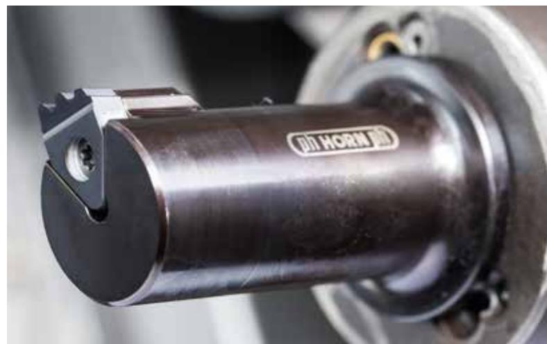
Standard cutting insert from the S117 system, with three cutting edges for pre-cutting and finish-cutting. A total of 55 strokes, each with an infeed of 0.1 mm (0.0039").
