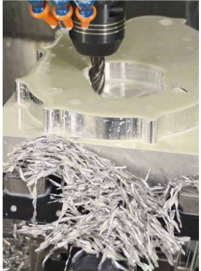
This example of trochoidal machining shows an aluminium block being machined with a contact depth of 20 mm (0.7874").
