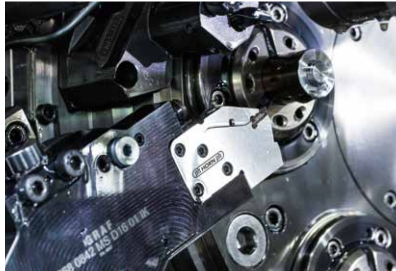
Cartridge and indexable insert from the 968 modular parting-off system.
