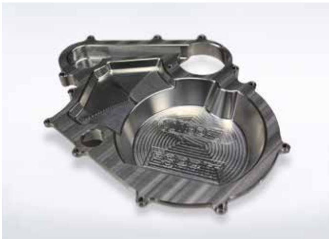
The finished casing component mainly undergoes trochoidal rough machining.
