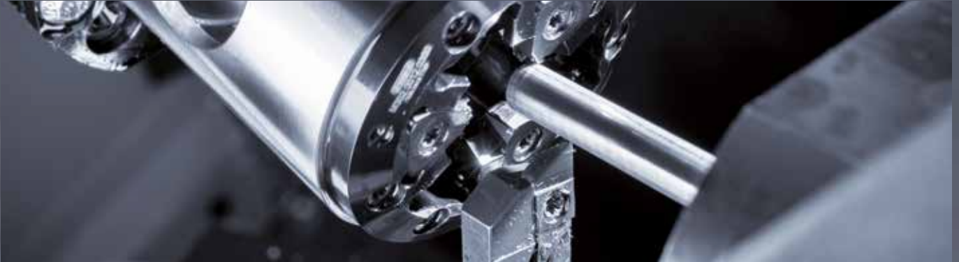
Rotary whirling in action: turning and whirling in parallel.
