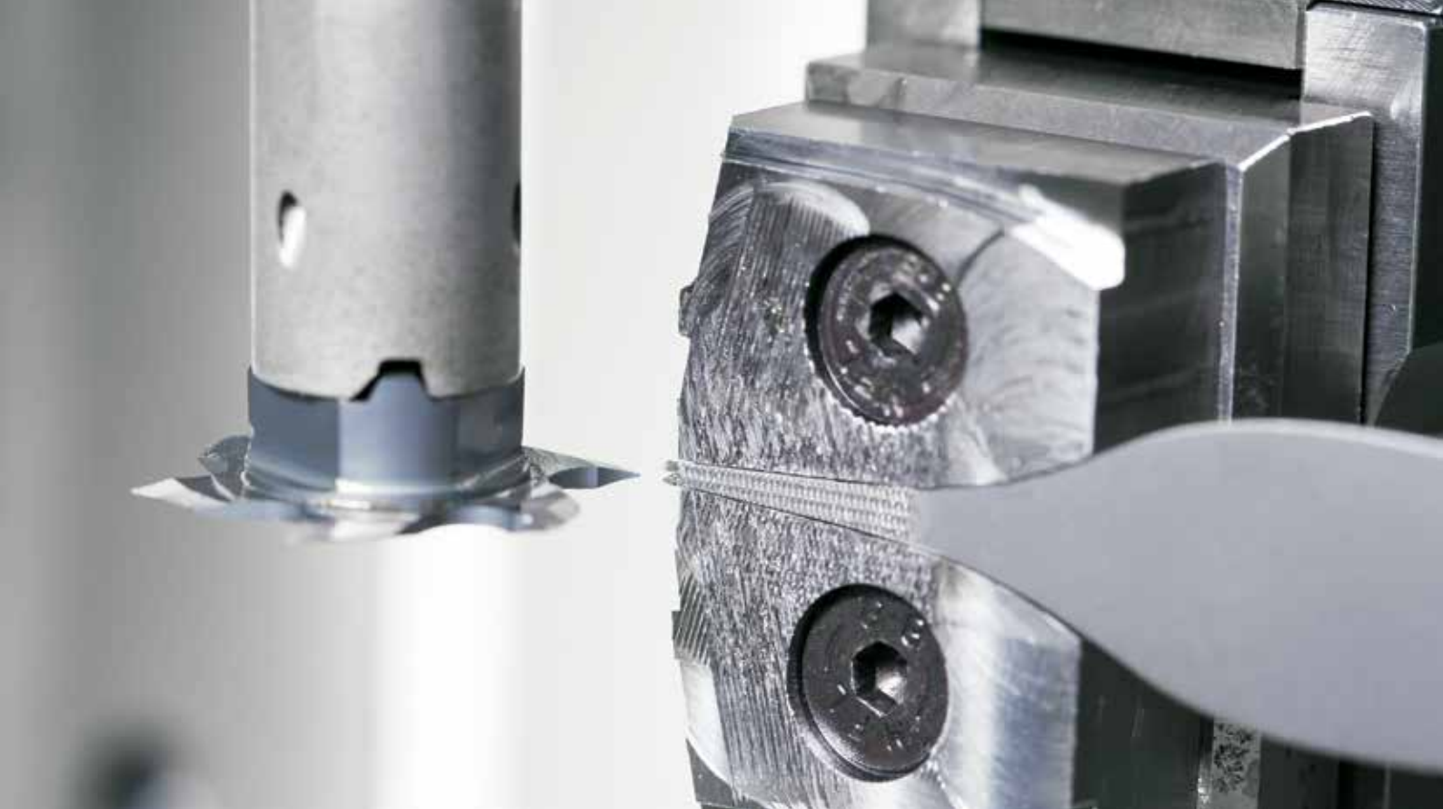
Cutting the female mouse tooth geometry. The flank angle of the profile is 25°, 30° or 35°, depending on the profile height.
