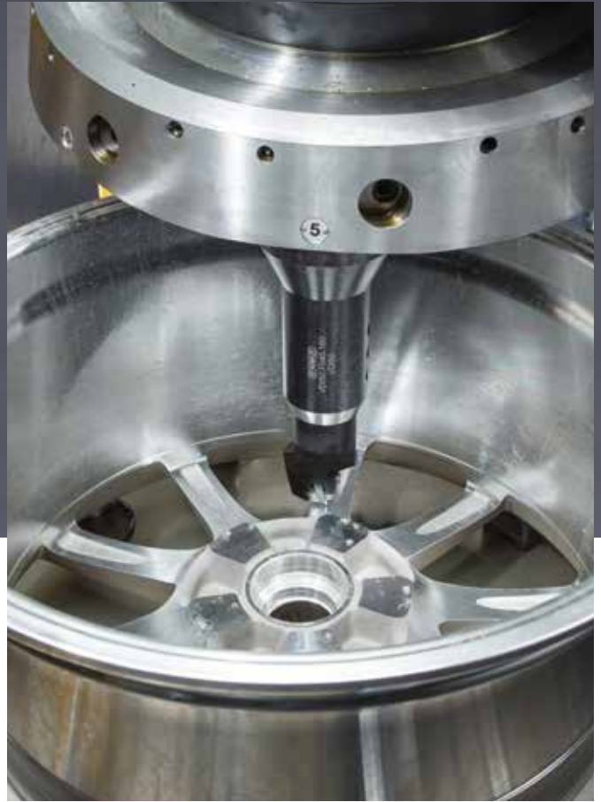
Turning the spokes with interrupted cutting.
