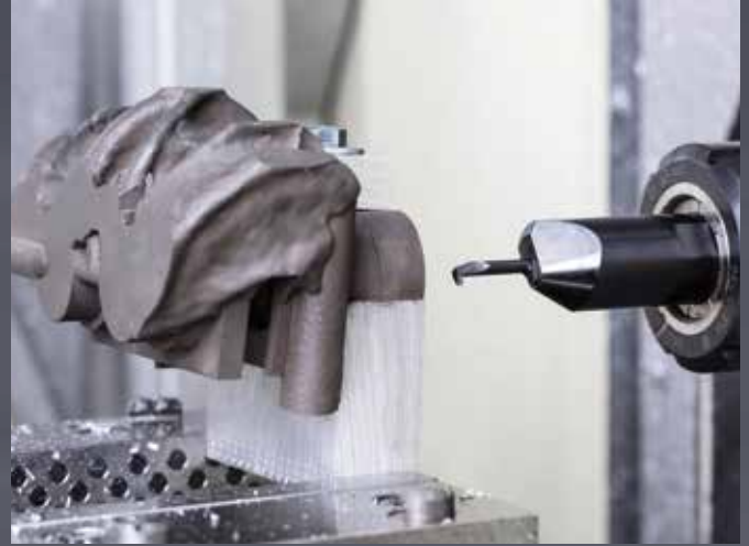
Finish boring a brake calliper with a Supermini 105.
