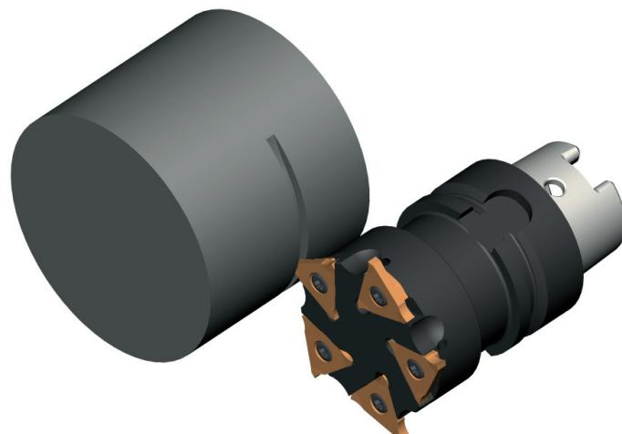
$$\cos \varphi^\circ = \frac{r^2 + [R + r - a_r]^2 - R^2}{2r[R + r - a_r]} \rightarrow \varphi^\circ$$
