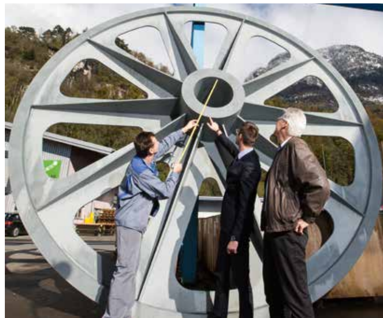
Cableway pulley with a diameter of 6 metres (236.2205"). Although Edi Hurschler (left) from Großbearbeitungs AG sees this impressive size as perfectly normal, the same cannot necessarily be said of Christian Thiele from HORN (centre) and Wilfried Iseppi from Dihawag (right).
