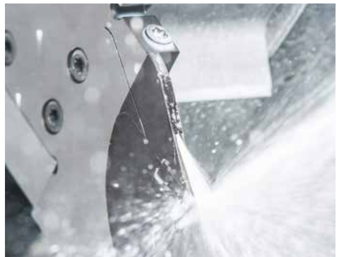
845 cartridge with internal cooling via the clamping finger and support cooling from below.
