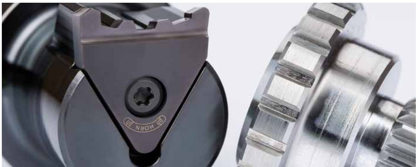
SH117 tooth broaching tool with pre-cutting and finished tooth profiles for simultaneous rough broaching and finish broaching of the teeth.
