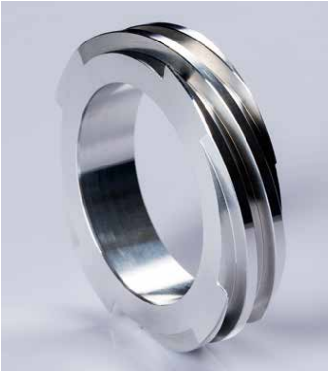
The finished workpiece with a quadruple square thread.
