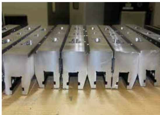
Picture left: After 23 clamping elements, the tools used for rough-milling are changed to ensure process reliability.
