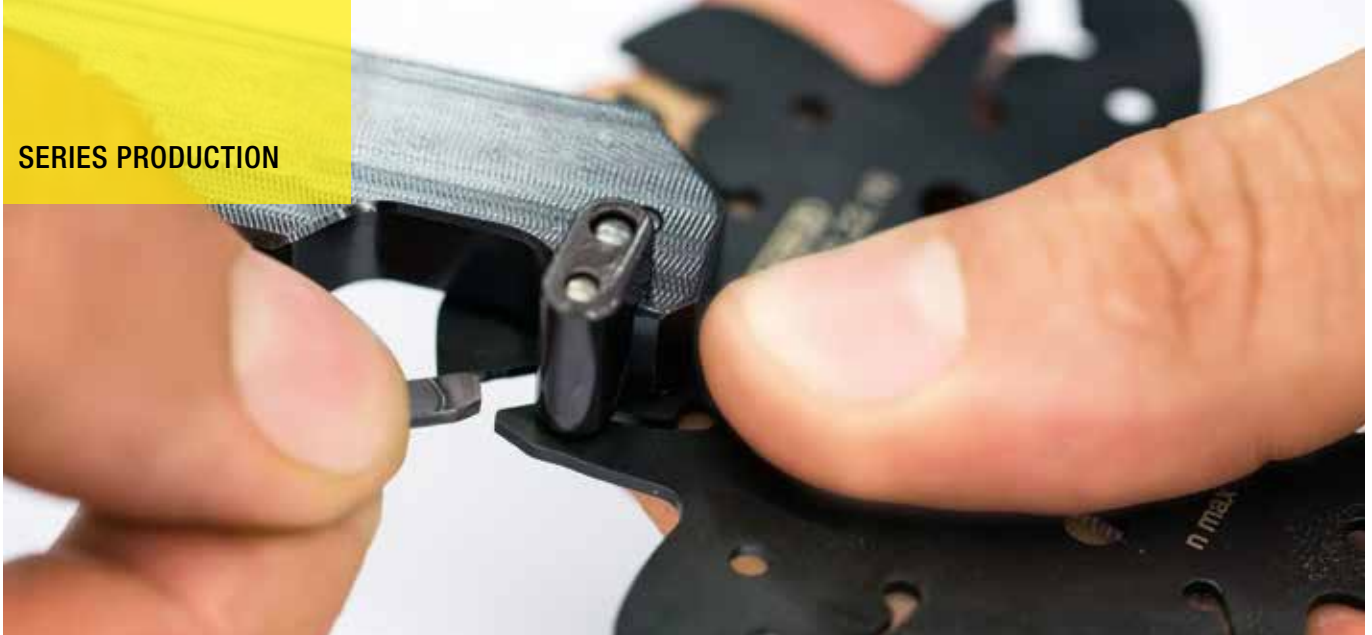
Lifting the clamping finger with a self-locking installation wrench. The stroke is restricted to a minimum. Both hands are left free to replace cutting inserts.
