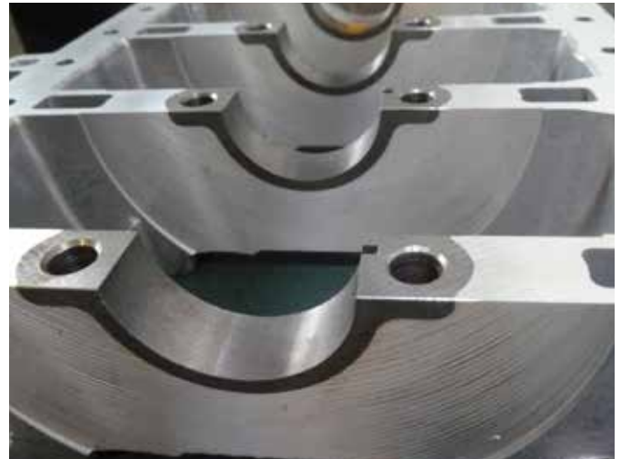
GGG60 bearing shells, in the form of half-shells cast in aluminium, combine to form a base and cover that create the crank shaft bearing.
