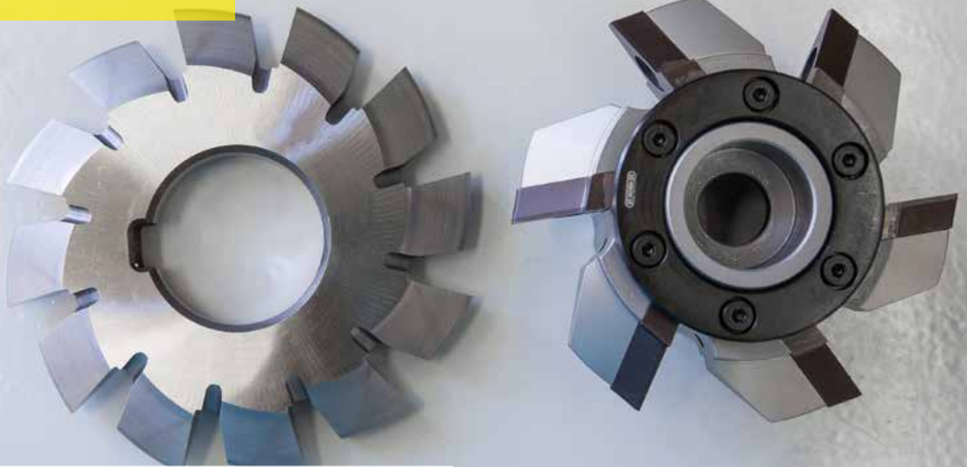
The M121 module milling cutter from HORN, equipped with six carbide cutting inserts, brilliantly took over from the previous HSS milling cutter.
